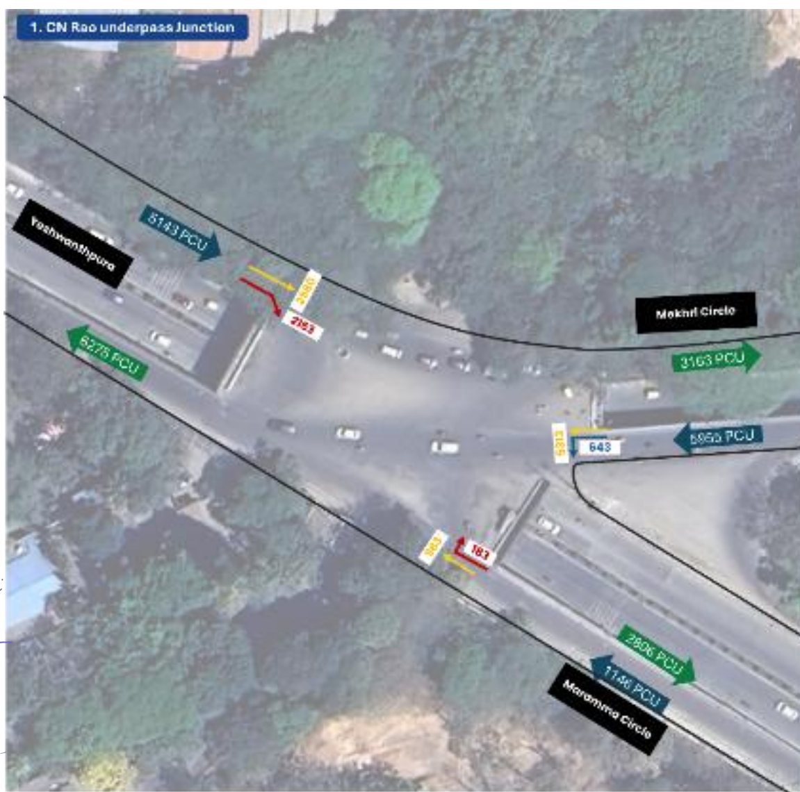
Figure 95: TMC at CN Rao Underpass Junction
